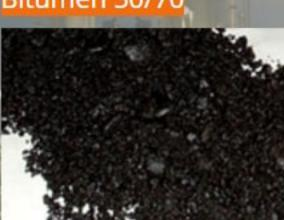
Bitumen Penetration Grade 50/70 is a standard penetration grade Bitumen usually used as a Paving Grade Bitumen suitable for road construction and for the production of asphalt pavements with superior properties.
