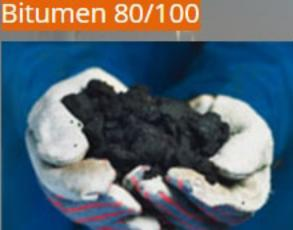
Bitumen Penetration Grade 80/100 is a standard penetration grade Bitumen usually used as a Paving Grade Bitumen suitable for road construction and for the production of asphalt pavements with superior properties.
