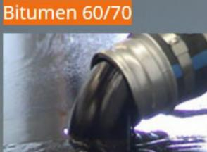
Bitumen Penetration Grade 60/70 is a standard penetration grade Bitumen usually used as a Paving Grade Bitumen suitable for roadconstruction and for the production of asphalt pavements with superior properties.
